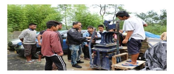
The resorce person MR.V .lyngdoh demonstrated the art of mudblock ,hollow block, and improved chullah making to the trainees to take it as an business activity .The ratio of mixing of sand and cement is in the ratio of 1:20 which is the essential components needed to hold the mixture together and the mixture is then put under pressure of the block cement machine to stabilize the components .
